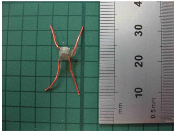
**Figure C.7:** Composite PTC-R nitrogen level sensor covered in epoxy.
