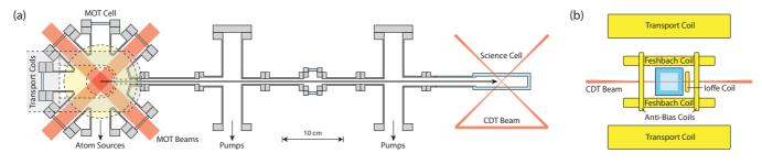
FIG. 1. (Color online) Outline of the experimental system. (a) Horizontal cross section through the vacuum chamber. Atoms are transported from the MOT cell to the science cell by the transport coils, mounted on a mechanical translation stage. (b) Region around the science cell as viewed down the transportation axis, showing the geometry of the coils used to create the QUIC trap and to access Feshbach resonances.
